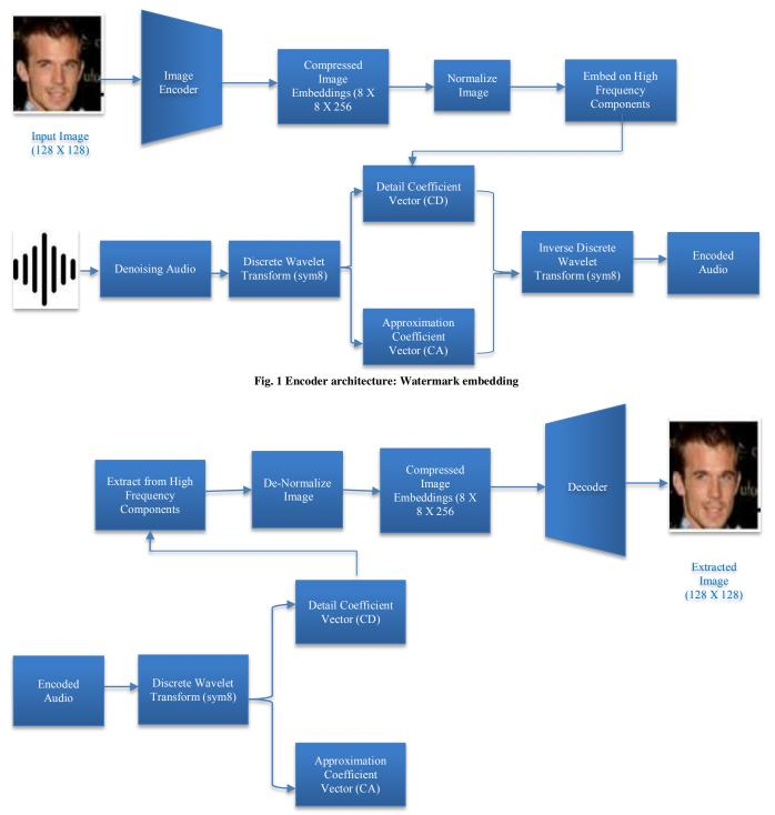
Fig. 2 Decoder architecture: Watermark extraction
