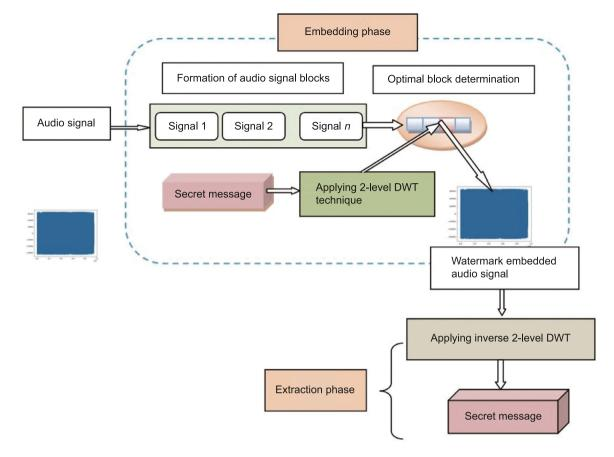
Fig. 1. Flow diagram of proposed digital audio watermarking based on search location optimization.
