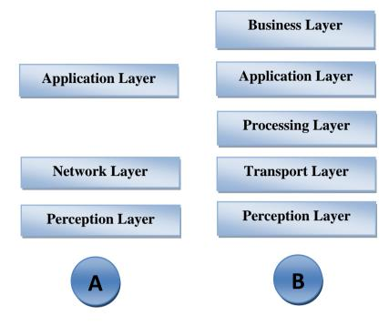
Figure 1.2: Three(A) and Five-Layer(B) Architectures (Lai, 2021)
