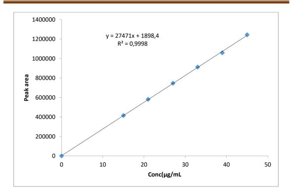
Fig. 6.9: Linearity Plot of Ritonavir
