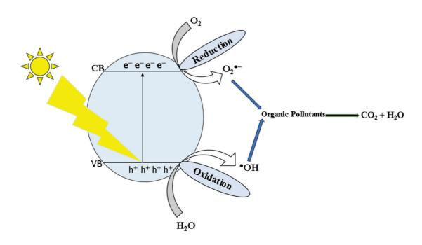
Fig. 1.2 Mechanism of Photocatalysis
