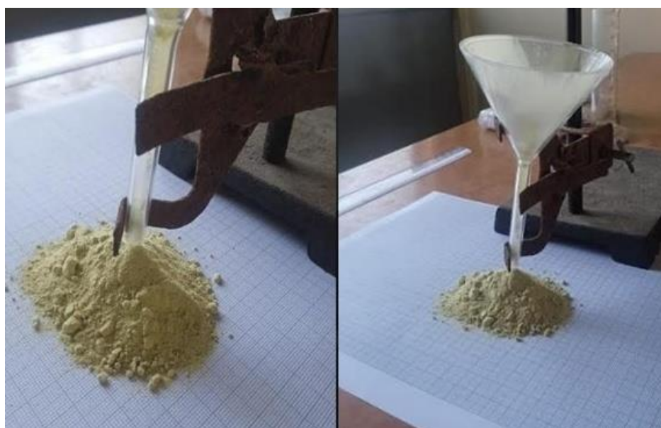
Figure 6.62: Angle of repose of PHF powder
