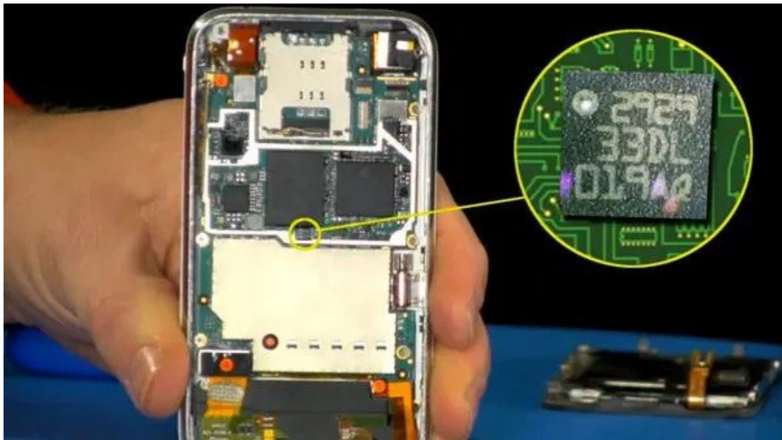
Fig. 1.6 : Magnified view of an accelerometer chip on a mobile phone motherboard
