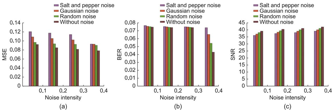
**Fig. 6.** Performance analysis for image 1 based on noise intensity. (a) MSE. (b) BER. (c) SNR.
