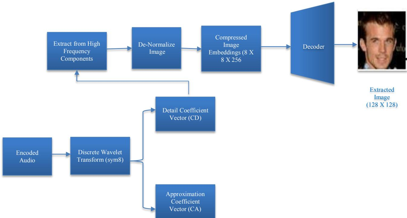
Fig. 2 Decoder architecture: Watermark extraction
