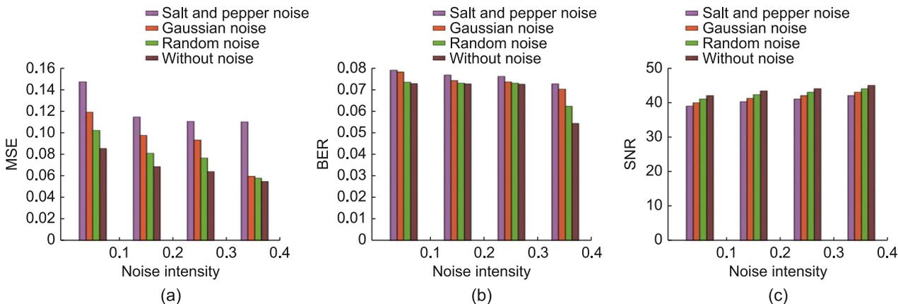
**Fig. 8.** Performance analysis for image 2 based on noise intensity. (a) MSE. (b) BER. (c) SNR.
