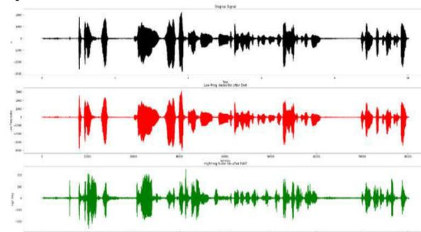
**Fig 3:** Audio Signal before applying DWT.(Color codes used : Black- Original Audio, Red-Low Frequency Component, Green-High Frequency Component.)
